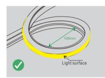
Light surface upwards, the strip is bendable to right or left naturally, the minimum bending diameter is 100mm.
