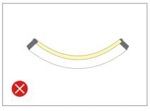
Face to the side surface(as the picture shows). Do not bend upward to damage the strip.
