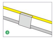
Fix led strip completely into the fixed clip, LED strip subface must be parallel to the top edge of fixed clip.
