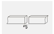
Make precise vertical cuts at the exact cut position of the light strip.
