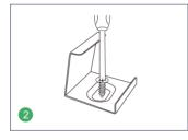
Adjust the fixed clips to theappropriateplace, use a screwdriver to fix the screw.
