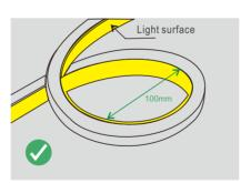
Light surface upwards, the strip is bendable to right or left naturally, the minimum bending diameter is 100mm.
