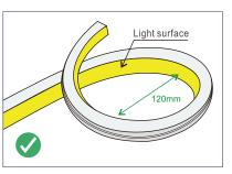
Lighting inside as above. Circle bending minimum diameters is 120mm.
