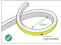
Lighting outside as above. Circle bending minimum diameters is 120mm.
